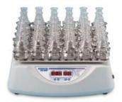
Flask Clamps (for SI-1600) are of stainless steel construction for added strength and safety. Mix and match different size clamps on same platform or all same size (capacity is indicated). Includes mounting screws. Note: Flask Clamps can also be used on SI-1700 by removing the blue Adhering
